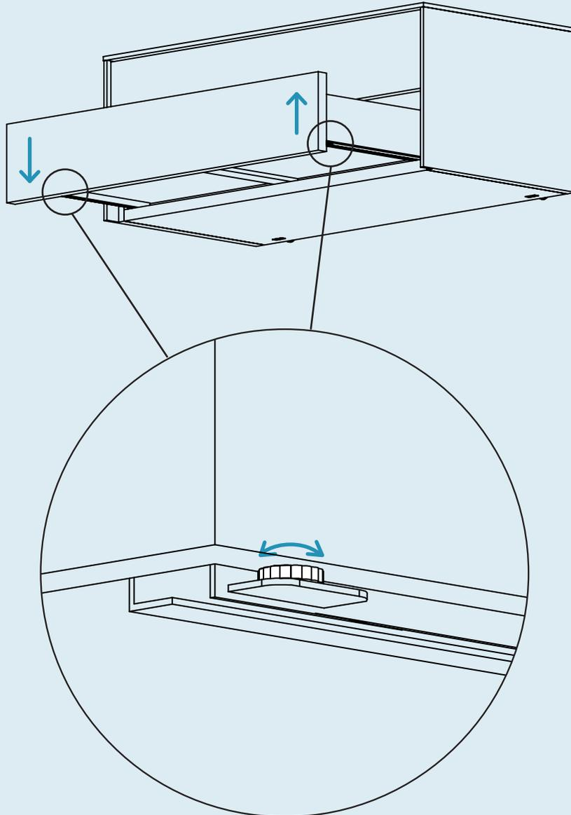
To lower the drawer as shown, turn the dial counterclockwise to lower the dial height.
